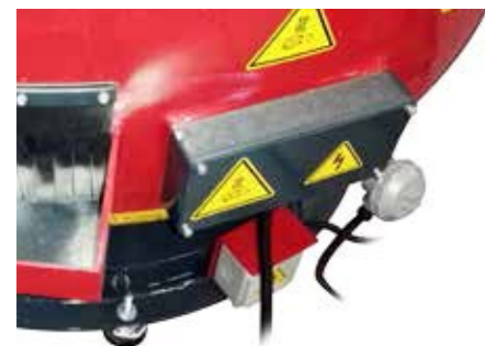
Resistance - electrical box with thermocouple.
