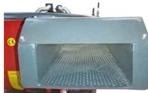
Inside of the unloading unit.
