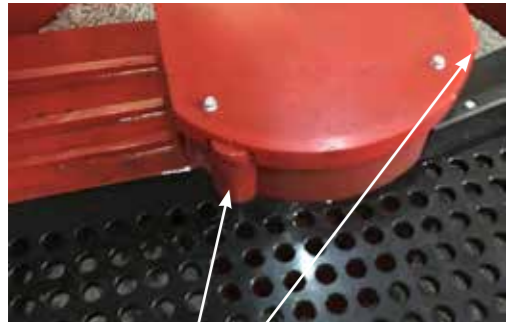
Easy changable screen with PU bumpers.
