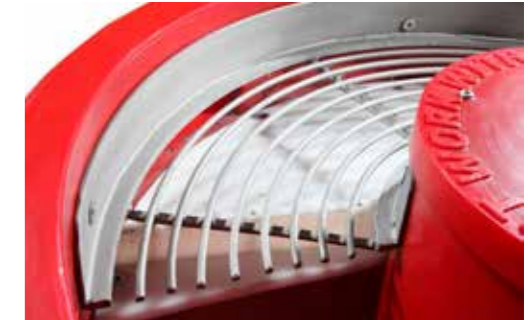
DL series, optional double layer screen unit.
