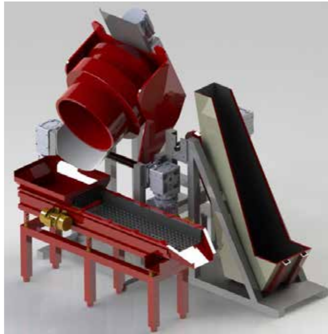
LOADING BUNKER - KSM160 - SM160
